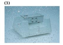
The aluminum load cell of the SJ-WP/SJ-WP-BT series is treated with alumite and silicon to be anti-corrosive and withstand long-term use in wet environments.
